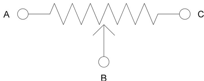
A rheostat works by varying the position of the “wiper” connected to terminal B. This position is often moved by turning a shaft. Notice that as the wiper position changes, the resistance from A to B and from B to C also changes, while the resistance from A to C remains the same. The resistances  $R_{AB}$  and  $R_{BC}$  can vary from 0 to  $R_{AC}$  and are related by the equation
