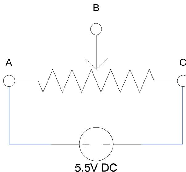
14. Set the wiper to make the voltage drop across terminals B-C of the rheostat to be 1.5 V (label your assumed voltage polarity). Calculate what resistance between terminals B-C is required to obtain the 1.5V drop. Verify your answer by disassembling your circuit and measuring the resistance directly.
