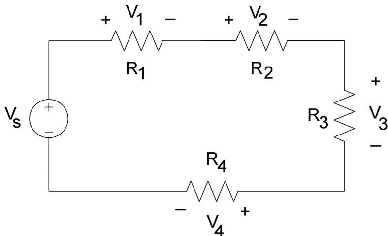
Figure 1. Series Circuit with Four Resistors
