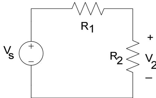
**Figure 2. Series Circuit with Two Resistors**
