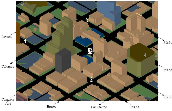
Fig. 2. A mobile communications system which consists of a base transceiver station and four mobile stations in the urban vehicular environment of downtown Austin, Texas. (MS 4 indicated here is behind the building on 8th Street.)
