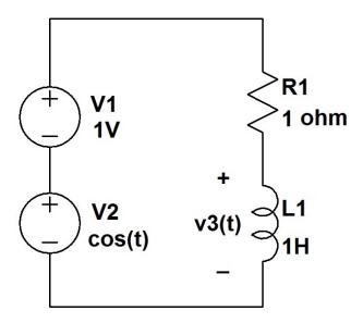
6. (5 points) Find node voltage v(t) in the sinusoidal steady state using nodal analysis.
