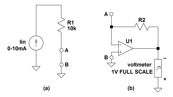
2. (5 points) Thevenize the following circuit "looking into" terminals A-B. Be sure to sketch the Thevenin equivalent circuit.
