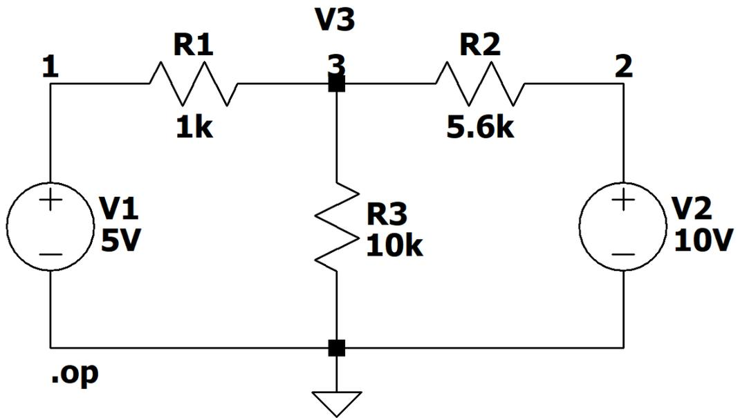
Figure 1. Circuit with Two Sources
