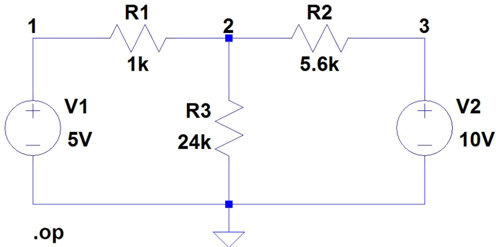
Figure 1. Circuit with Two Sources
