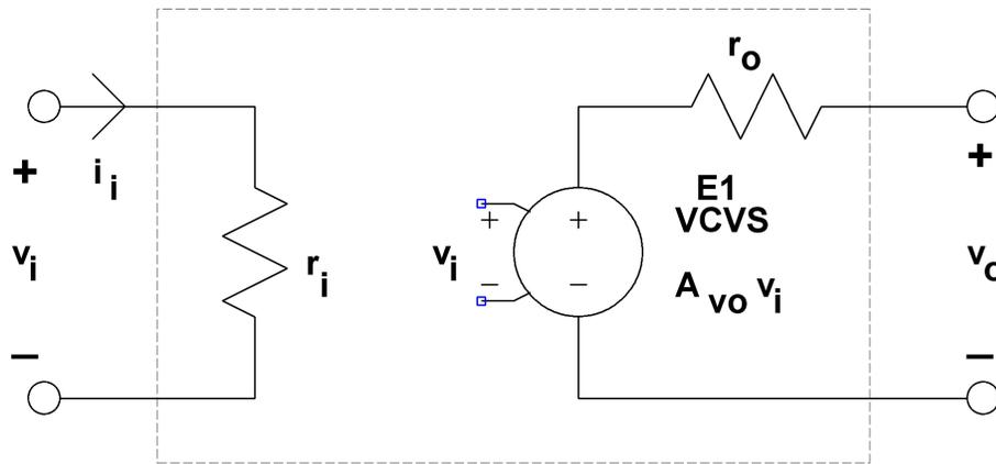
Figure 1. Small Signal Amplifier Model
