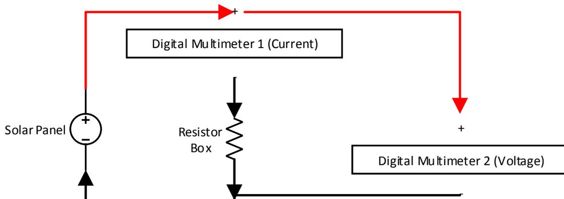
**Figure 4: Electrical Circuit in Part 2**
