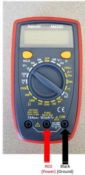
**Figure 2: DMM in the 20V Position**
