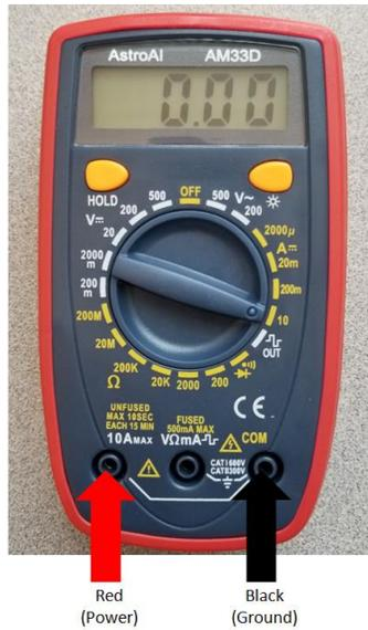
**Figure 3: DMM in the 10A Position**
